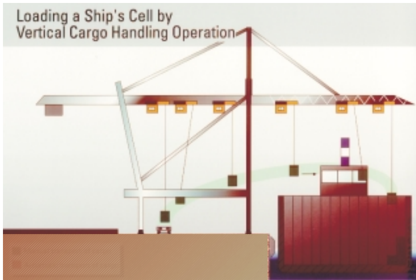
Figure 1 Schematic drawing of the container crane and its trajectory of the container.
