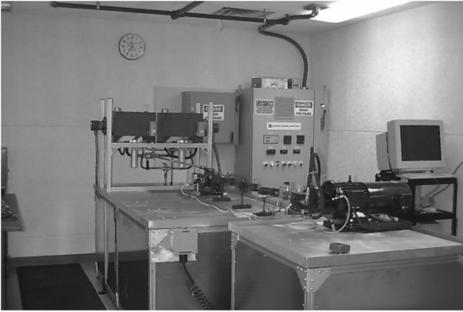
Fig. 1 Experimental set-up for testing pumps
