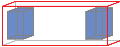
(a) Large inertia with the mass away from CG
