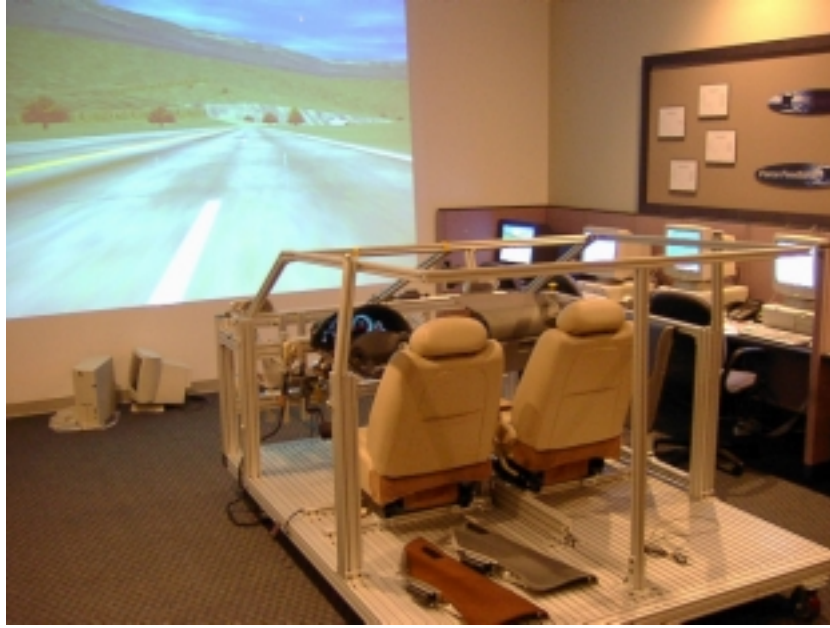
Figure 4: The Virtual Vehicle Systems Simulation Laboratory consists of a human-in-the-loop driving environment with MATLAB/Simulink-based workstations for modeling and design.
