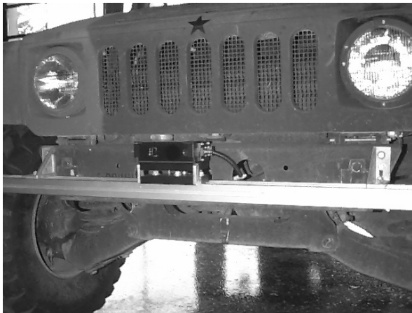
Figure 1 Laser radar sensor mounted on the front bumper of a US Army HMMWV
