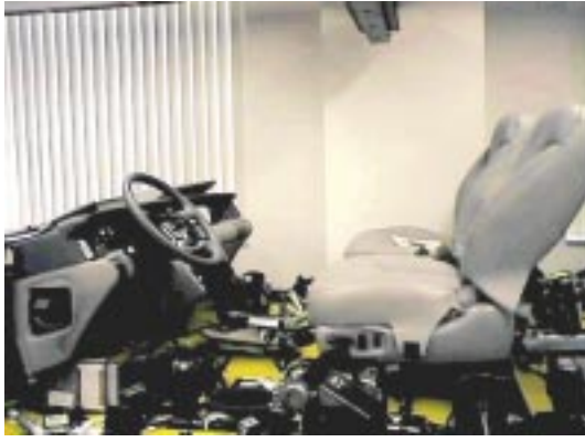
Figure 4: The user interface is implemented as a full driver cabin.
