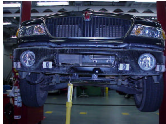
Figure 1 Four radar units in front of the bumper
